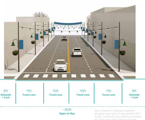
generally have rights-of-way between 60ft to 66ft. All arterial cross sections are shown for a 60ft-wide right-of-way to provide consistency. Rights-of-way wider than 60ft provide opportunity for wider sidewalks, bike lanes, and street terraces than shown
