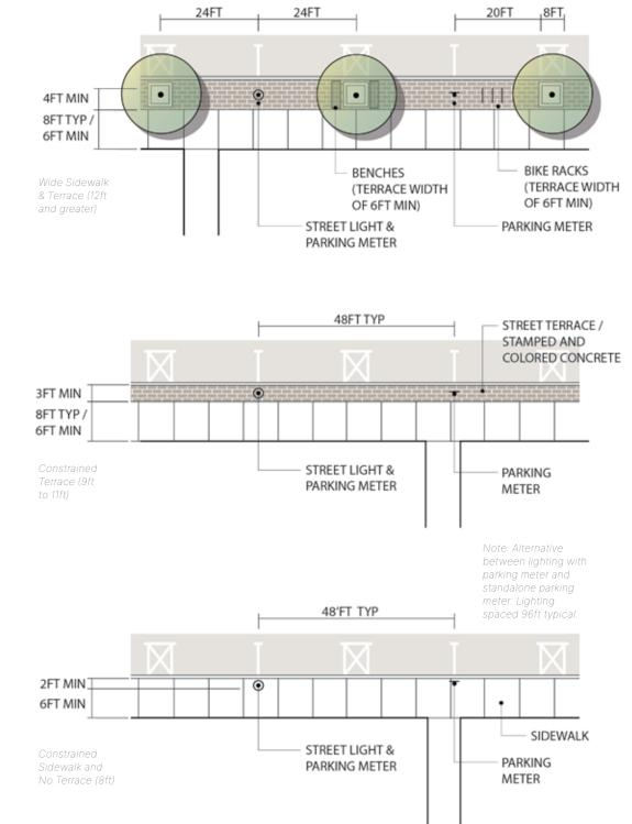
Sidewalks should be designed to provide a safe and accessible pedestrian experience. A minimum width of 8ft and minimum clear space (no light posts or other obstructions) of 6ft is recommended for all sidewalks.
