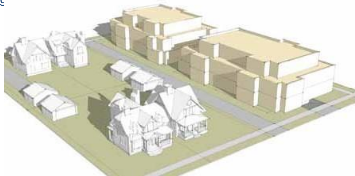
Figure 72 Stepping back upper stories and articulating the rear façade can reduce the overall mass and scale of new development. This is especially important in transitional mixed use
